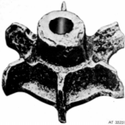
Figure 2-7. Corrosion of water pump impeller.
